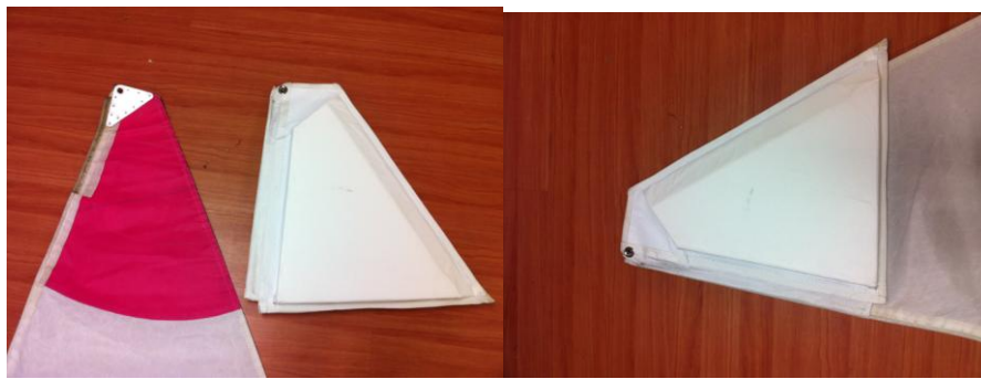
The masthead float is made with 1.5-inch foam in a sleeve secured over the head of the sail.
